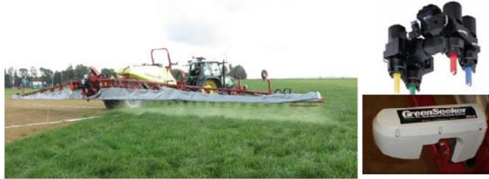
Fig. 25.8 Varioselect ® nozzle holder ( upper right ) and GreenSeeker ® sensor placed on the spray boom ( bottom right ), sprayer sprays a high volume above green grass ( right in left picture .) and a low volume above desiccated grass ( left )
